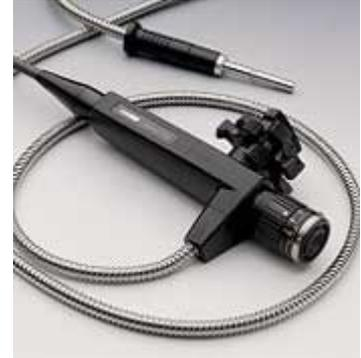
**Interchangeable optical tip adaptors.** The focus of the optical system is fixed, however, each inspection has different requirements with regard to depth of field and direction of view. For this reason, all standard model fiberscopes have interchangeable optical tip adaptors to provide versatility and are available in direct or side viewing configuration - just select the tip adaptor most suitable for the application. Separately, a diopter focus compensates for the individual's eyesight.
