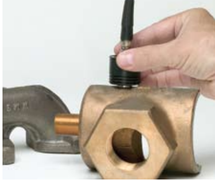
Cylinder bores and many other cast metal parts or sound-attenuating materials can be measured with the 35HP gages.
