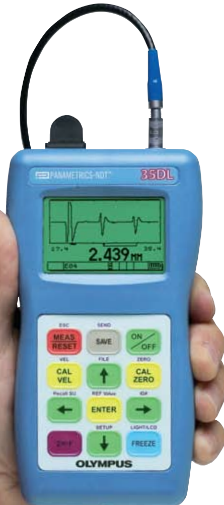
You can measure critical thickness metal thinning caused by bending.
