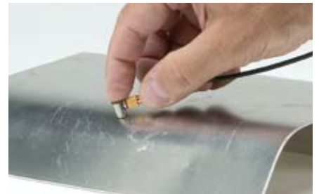
You can measure critical thickness metal thinning caused by bending.
