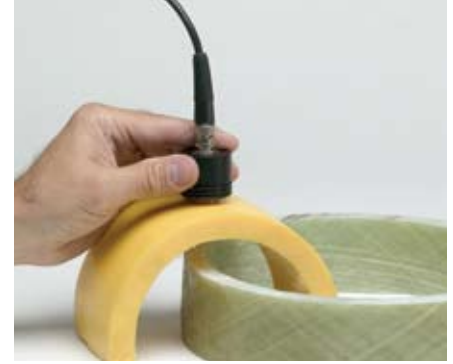
The 35HP gages are excellent tools to measure fiberglass or composite parts, from aerospace structures to boat hulls and storage tanks that require thickness control.
