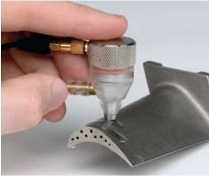
The Model 35 with a delay line transducer or immersion bubbler makes accurate thickness measurements on both convex and concave surfaces of turbine blades.
