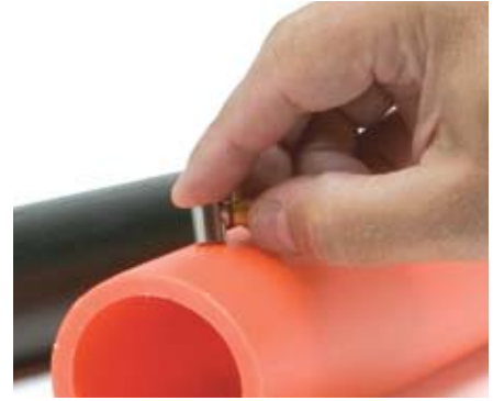
Plastic or metal tubes and pipes of various diameters can easily be measured ultrasonically with contact type transducers. Small diameters may require immersion type measurements.
